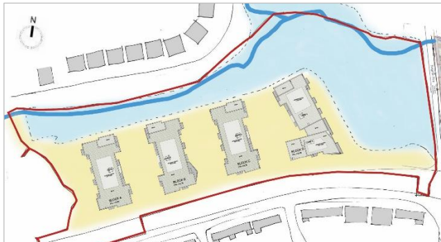
Fig. 3.0.1 Indicative illustration showing how the design rationale is informed by the flood zone.
